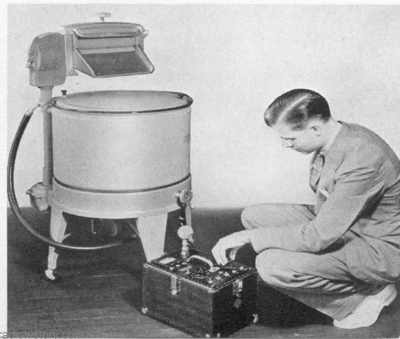
FIGURE 4. The washing machine is only one of the many home appliances which the sound-level meter has helped to make quieter
